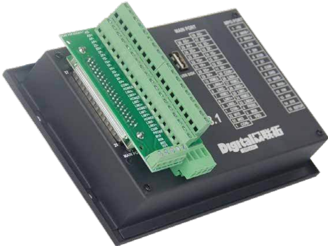
Figure 2-8 Main Port with wiring terminal
